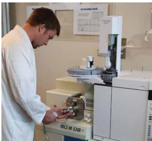
Brad Lewis operates the accurate-mass time-of-flight spectrometer, which can rapidly identify the presence of chemicals of interest. Photo: G. Vaughan, OEH.
